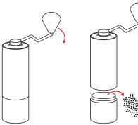
Cover the handle and hold the body tightly Rotate the handle clockwise to grind into powder
